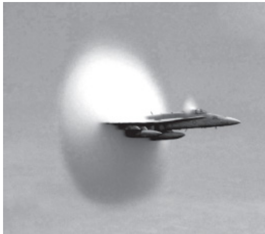
Figure 5.8. Vapor cloud around an F/A-18 jet fighter flying at transonic speed. (U.S. Navy photo by Ensign John Gay)
